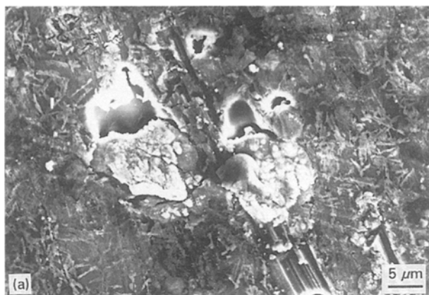
Figure 7 Molybdenum/aluminium alloy joint, fracture surfaces, (a) aluminium side and (b) molybdenum side, SEM.
